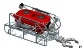
gure 1 - A CAD model of the Omega ROV
